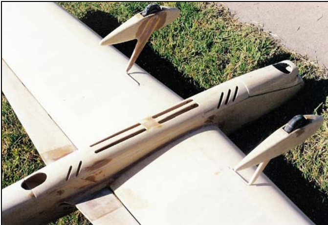
Yes, I use balsa wheel pants on ALL my stunters! Here they are on my "Special Effects" full fuselage pipe ship
