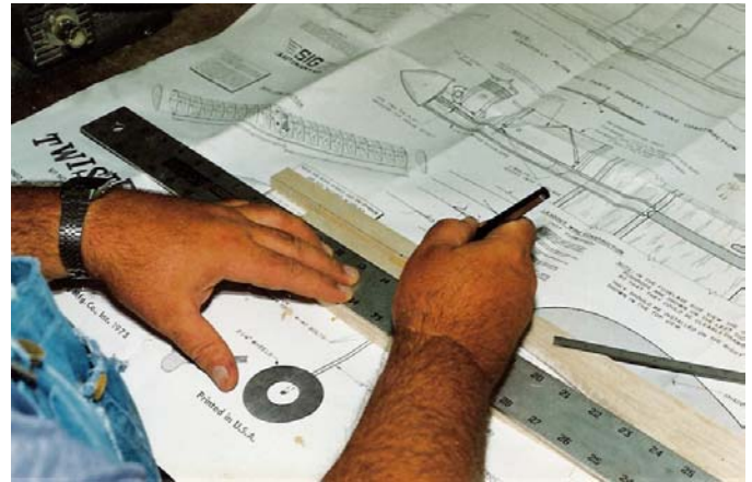
Drawing fuselage reference thrust line
