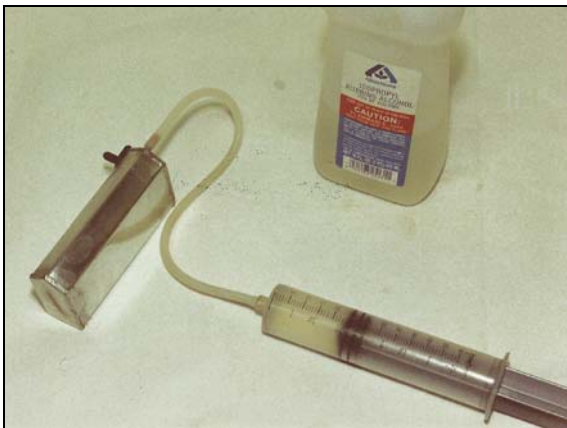
Cleaning and pressure testing the modified fuel tank
