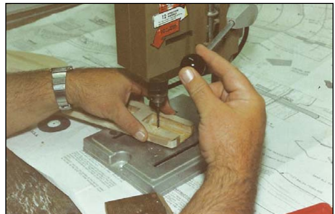
Precision drilling engine mounting holes
