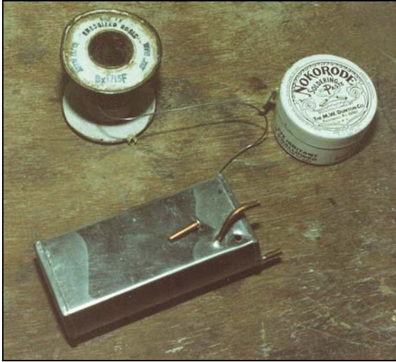
Metal fuel tank modifications for recessed mount
