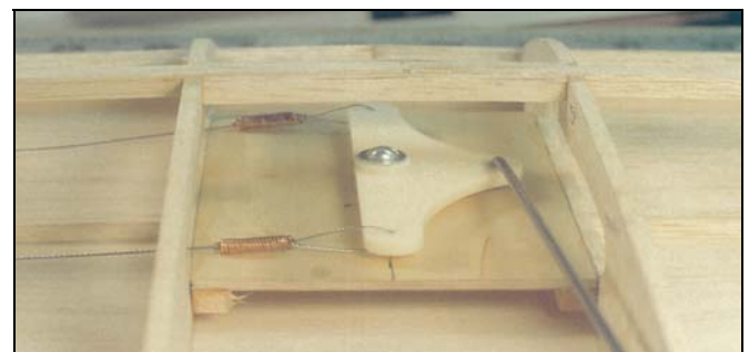
Copper wire wrapped leadout ends
